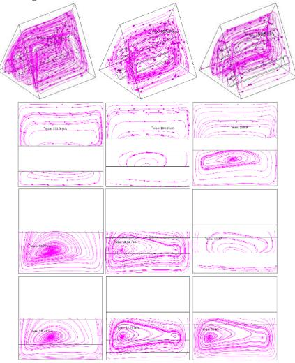
(a) Case2. (b) Case3. (c) Case4. Fig. 12. The streamlines at  $Ra=10^6$  and  $\phi=0.05$
