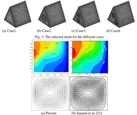
Fig. 4. The validation of the present data with Sannad et al. [31], isotherms (up) and streamlines (down)
