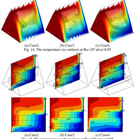
Fig. 15. The temperature isotherm lines at Ra= $10^6$  and  $\varphi$ =0.05
